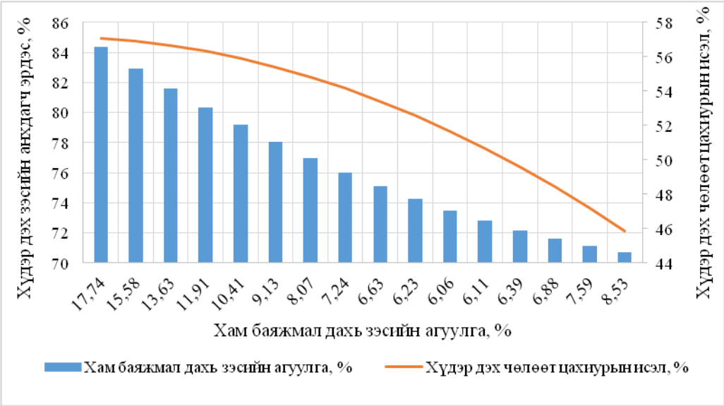
Figure 2 - Correlation between mineral content in ore and copper content in joint-concentrate
