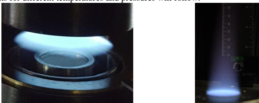
Figure 4 - Stabilized methane flame in counterflow burner (left, Z_{st}=0.1 ) and in heat flux burner (right, \phi=0.9 )
