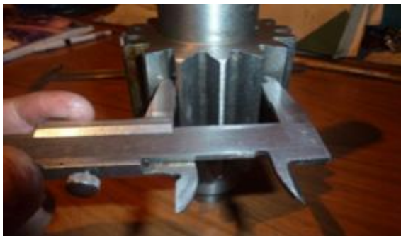
Figure 1: Checking the gear teeth "K" using a universal caliper
